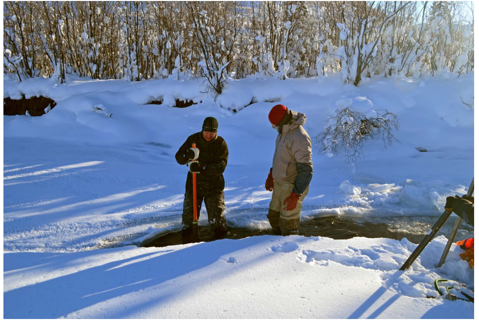
Installing water temperature data loggers in the Rat River, March 2013
